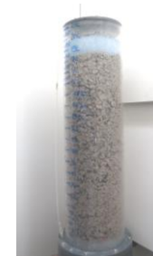
Percolate column leach test facility
